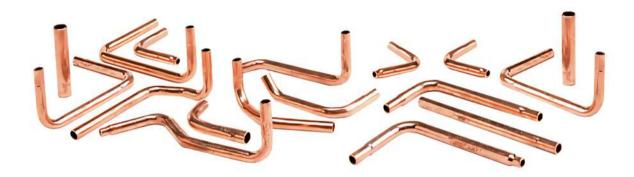
Briscool shapes Copper, Aluminum and Stainless Steel Tubes in a wide range diameter range from 2 mm to 32 mm, blows out and welds the elements necessary for use with cold soldering welding or induction machines. In accordance with the requirement, these pipes are subjected to 100% gauge control and flow and leak test.
